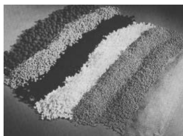
Figure 10-4a Catalyst particles of different shapes (spheres, cylinders) and sizes (0.1 cm to 1 cm). (Photo courtesy of the Engelhard Corporation.)
